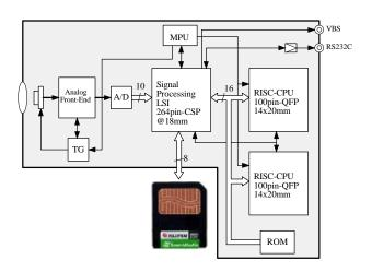
Figure 2. A Block Diagram for MX-600 ZOOM
