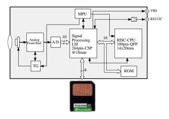
Figure 3. A Block Diagram For MX-500
