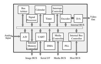
Figure 4. A Signal Processing LSI
